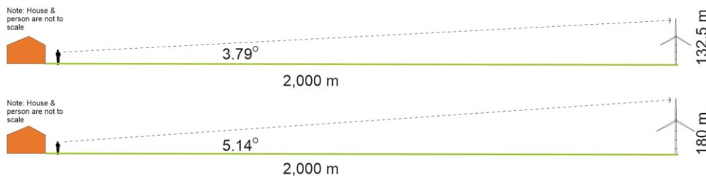
**Figure 1** demonstrates that the angle of view to a wind turbine of 132.5 m compared to the angle of view for a turbine that is 180 m high is similar. The viewing angle increases from  $3.79^\circ$  to  $5.14^\circ$ , an increase of less than  $1.4^\circ$  in the vertical field of view.
